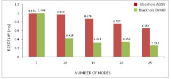
Fig: End To End Delay versus number of nodes
