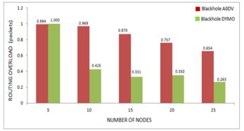
Fig: Routing Overload versus number of nodes
